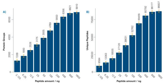
A) The TIMS XR allows for increased ion capacity for sample loads beyond 200 ng. Reproducible identification of ~ 6900 protein group identifications and more than 86,000 unique peptide identifications B) using the PaSER realtime search engine with TIMScore for dda-PASEF of up to 1600 ng K562 tryptic digest. Error bars indicate standard deviation for 5 replicates with mean displayed above histogram.
