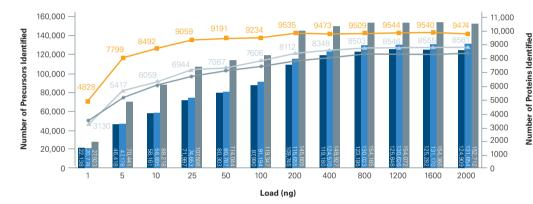
1 ng to 2000 ng of K562 material was loaded onto timsTOF HT run in dia-PASEF mode and searched with TIMS-DIA NN against a library made with and without TIMScore and Match Between Runs (MBR)
